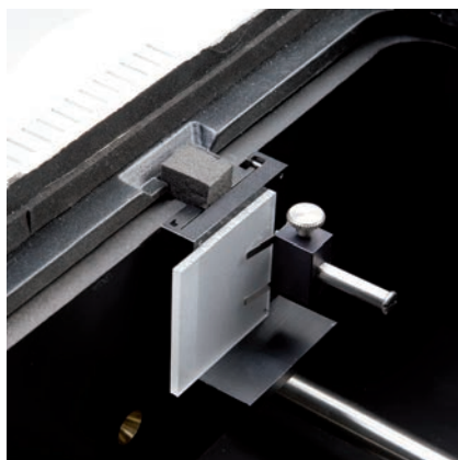
Solid sample holder to determine transmission characteristics
