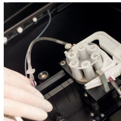
Sipper system for routine quantitative analysis
