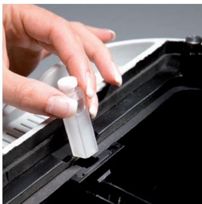
Dedicated position for turbid samples for measuring highly scattering samples
