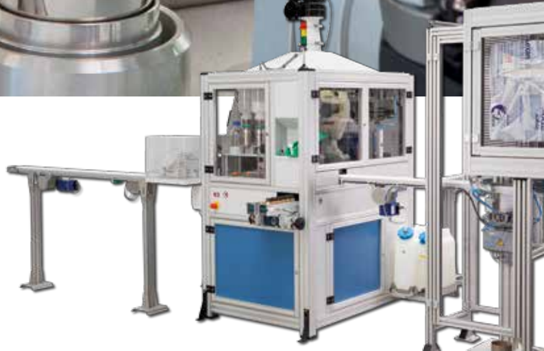
HAG-HF connected with conveyor belt to TGA (right) and spectrometer (left)
