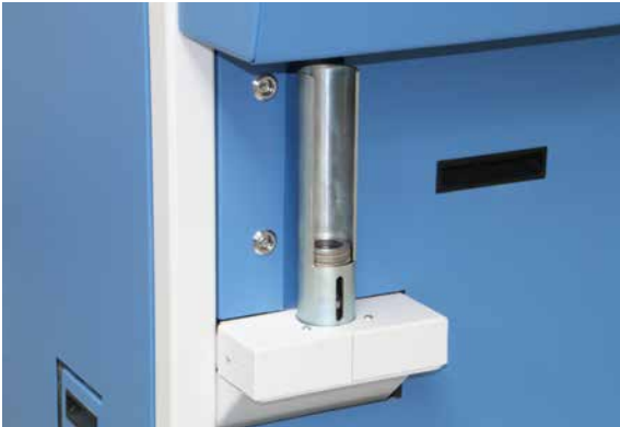
23-position ring magazine for clean and filled rings (option)
