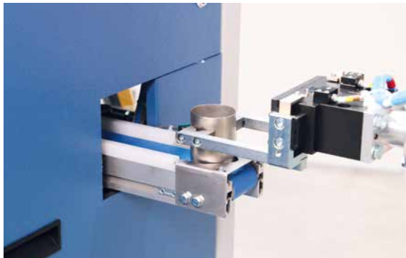
Various possibilities of sample input and output (here: sample input from the side by a robot)
