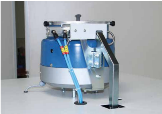
Dosing unit for grinding aid in tablet form (option)
