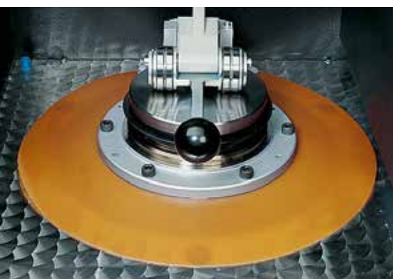
HSM 100 H with manual clamping device
