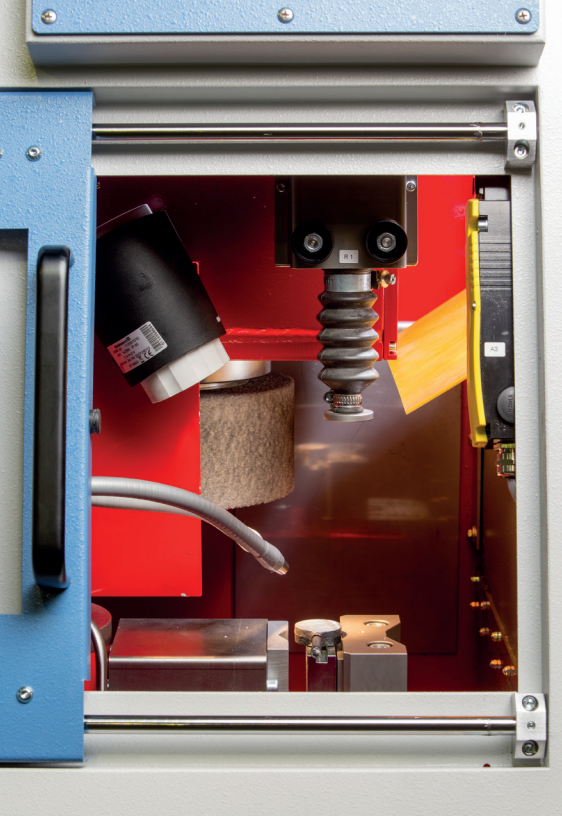
HTS 2000 with hydropneumatic clamping device
