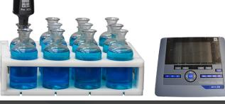
Manually prepare dilutions and place DO probe in bottles and BOD Pro<sup>™</sup> software will take care of the rest!
