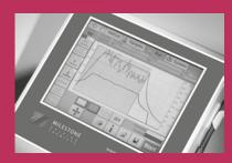
The synthWAVE is controlled via a compact terminal with an easy-to-read, bright, full-colour, touchscreen display. The terminal is provided with multiple USB and Ethernet ports for interfacing the instrument to external devices and to the local laboratory network.
