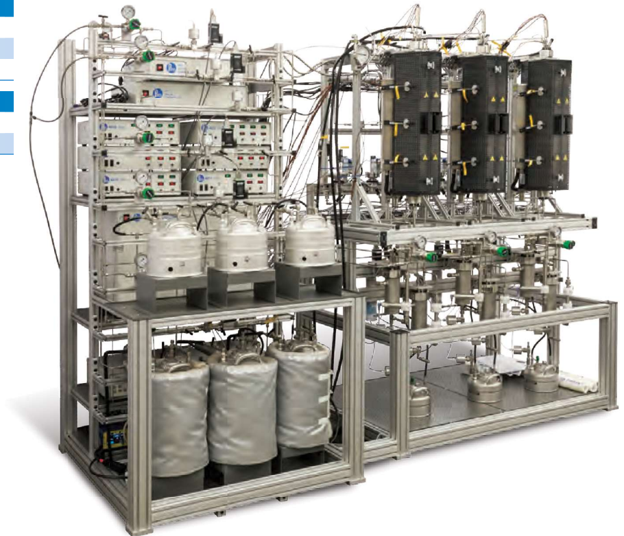
The system above has three 250 mL tubular reactors operating in parallel and controlled by a 4871 Process Controller with operator interface on a single PC. This system has weighed and/or heated feed tanks and a two-stage pressure let down.
