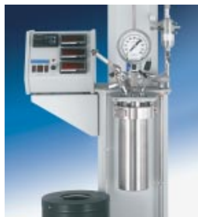
4534 Reactor, Assembled with Heater Lowered
